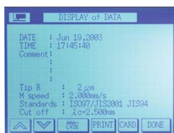
Display of all measuring conditions
