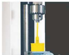
Insert test of plastic pipe
