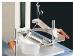
Peeling test of food contain cup
