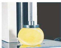
Compression test of tennis ball
