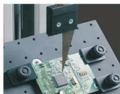
Soldering strength test of IC parts
