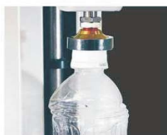
Compression test of plastic bottle
