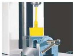
Insert test of plastic pipe
