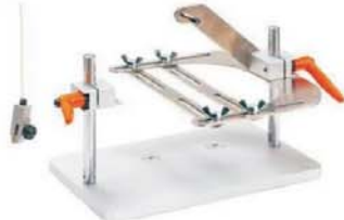
Peeling test of food contain cup
