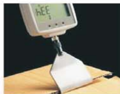
Opening strength of glued corrugated cardboard
