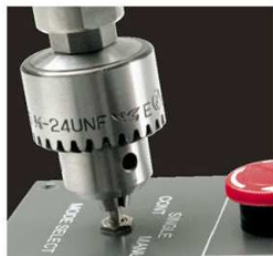
The example of the feeling measurement of a click of a rotary switch by HTG2.
