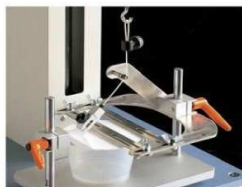
Peeling test of food contain cup
