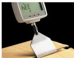
Opening strength of glued corrugated cardboard
