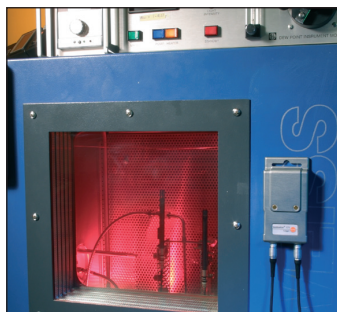
Monitoring air humidity/temperature fluctuations in climatic cabinet
