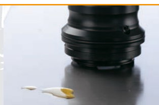
Measuring an oil film on steel
