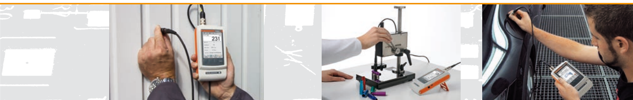
Measuring paint coating on steel
